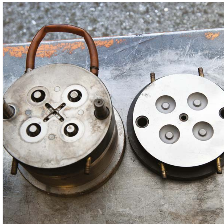
Tool for production of the first Polycom product - hygienic cigarette extinguisher
